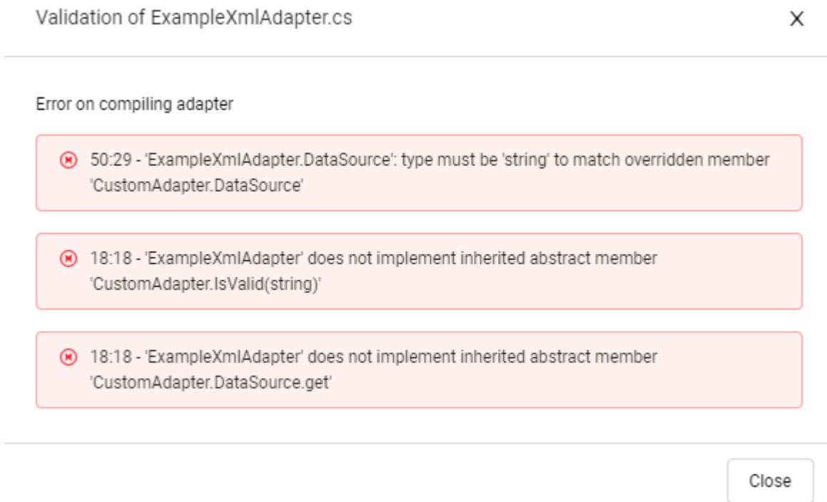
Figure 4.56: Compiling error messages on a failed import of a Custom Adapter
